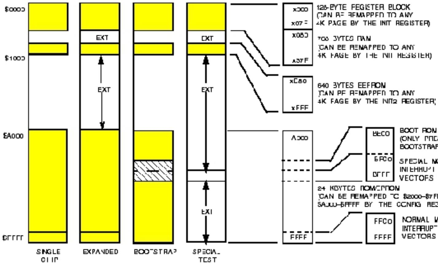
NOTE: POWERPROM CAN BE ENABLED IN SPECIAL TEST MODE BY SETTING POWEN BIT IN THE CONFIG REGISTER AFTER RESET
